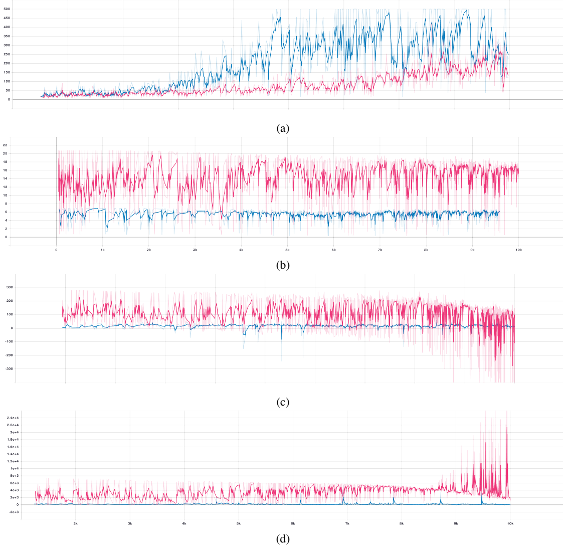
Figure 11: In this figure we switched gradient clipping on and off. (a) Shows the reward obtained by agent (b) shows the entropy (c) shows the policy loss (d) shows the value loss.
